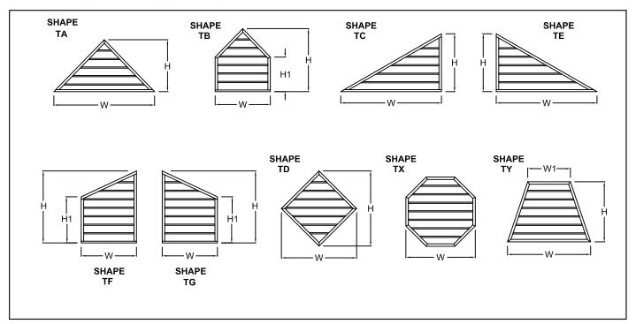
Note: Special shaped louvers are not AMCA tested for water penetration or air flow resistance. Conservative air flows should be used when sizing louvers to help prevent water carry over.
