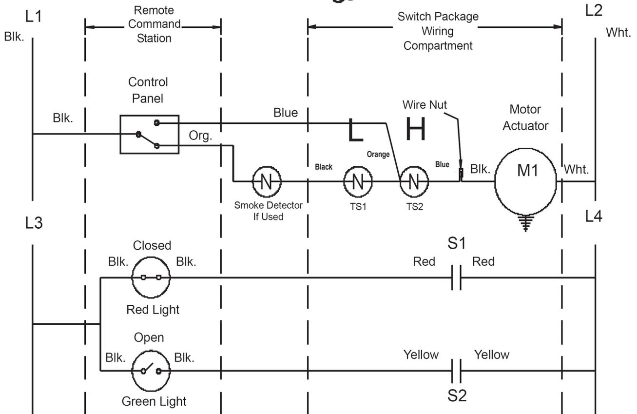
L3, L4 is a Supply Voltage Compatible with Lights and Switches. Standard Voltage is Same as Actuator Ordered.
